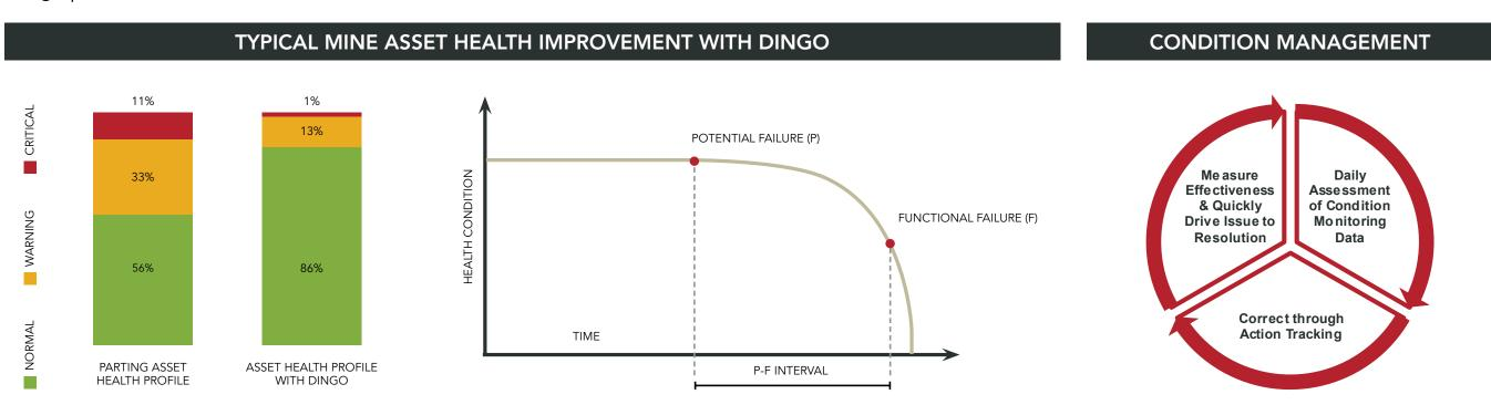
DINGO's Condition Based Component Change (CBCC) program helps site planning and reliability teams move from planned maintenance to changing out components based on condition. This customer example shows the savings on a haul truck fleet:
